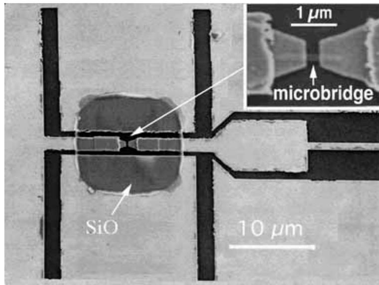
**Figure 5-10. Superconducting Nb hot electron microbridge bolometer mixer. This device extends high performance heterodyne receiver technology to 120 $\mu$ m, with future efforts pushing toward even shorter wavelengths. Its small size contributes to its ability to operate over a large spectral bandwidth. Thanks to JPL.**
