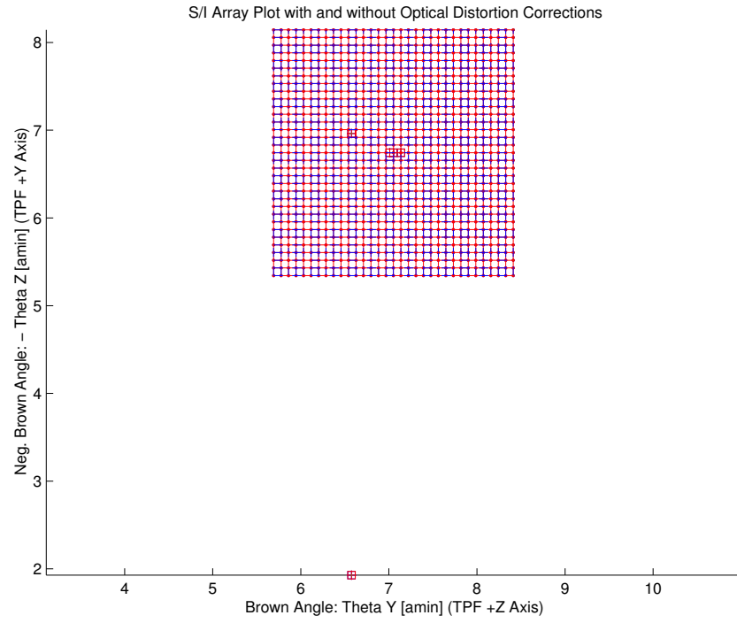
Figure 3.28: Array plot with (solid) and w/o (dashed) optical distortion corrections
