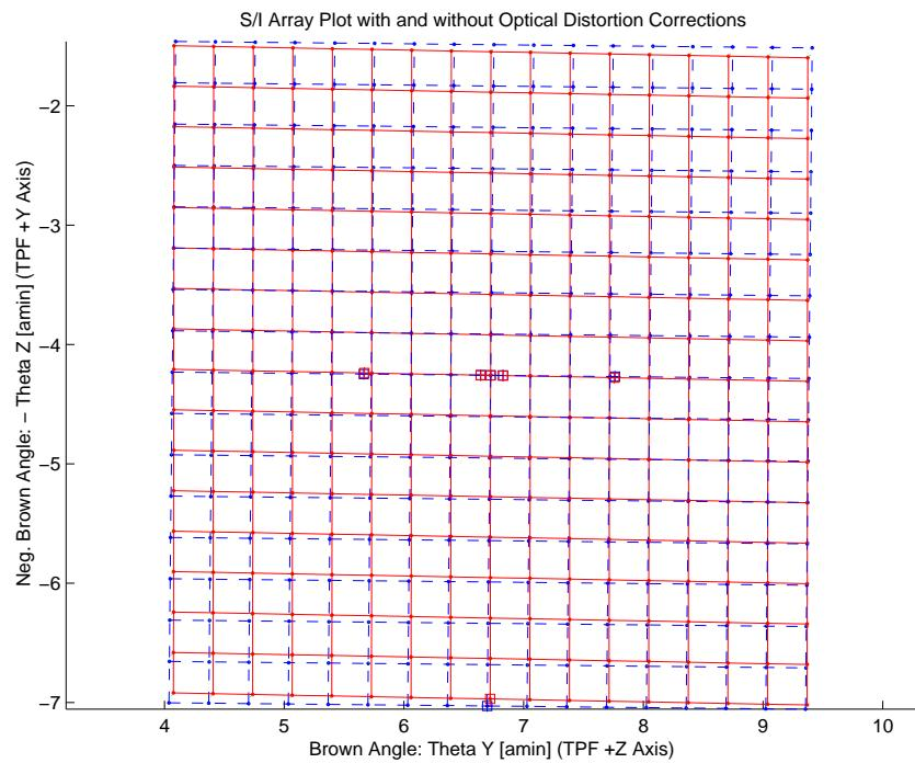
Figure 3.12: Array plot with (solid) and w/o (dashed) optical distortion corrections
