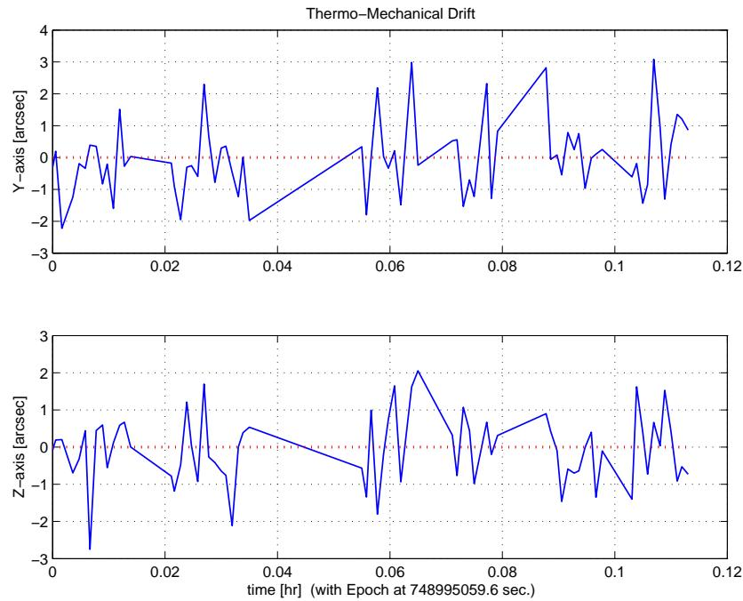
Figure 3.22: Thermo-mechanical boresight drift (equiv. angle in Body frame)
