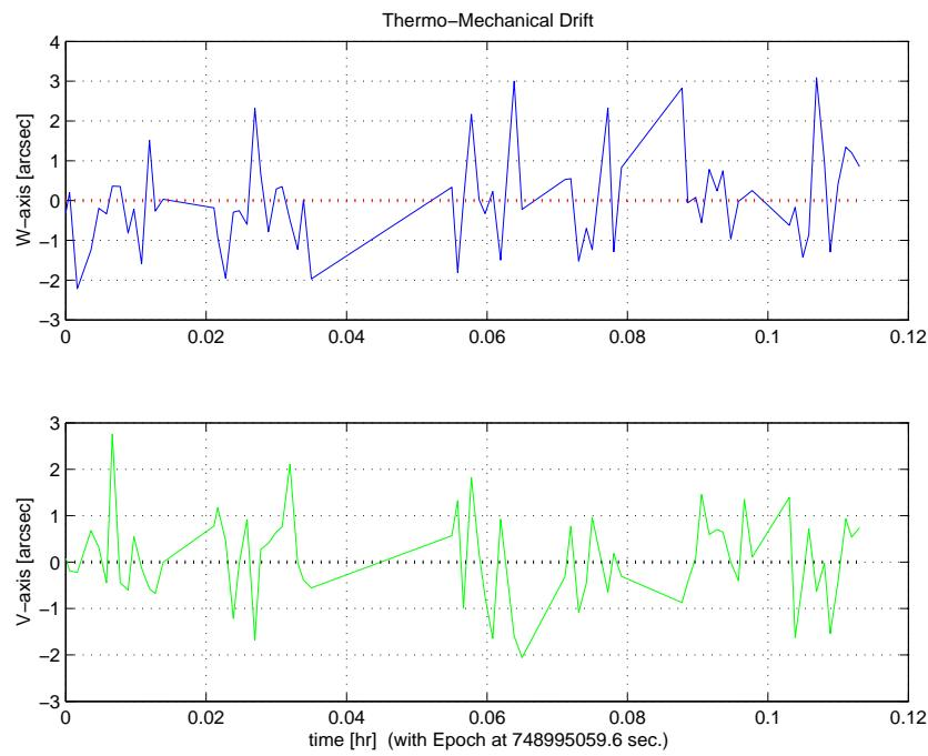
Figure 3.21: Thermo-mechanical boresight drift (equiv. angle in (W,V) coords)
