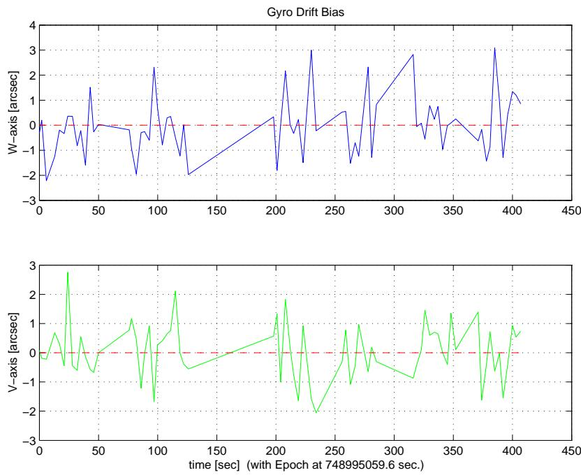
Figure 3.24: Gyro drift bias contribution (equiv. angle in (W,V) coords)
