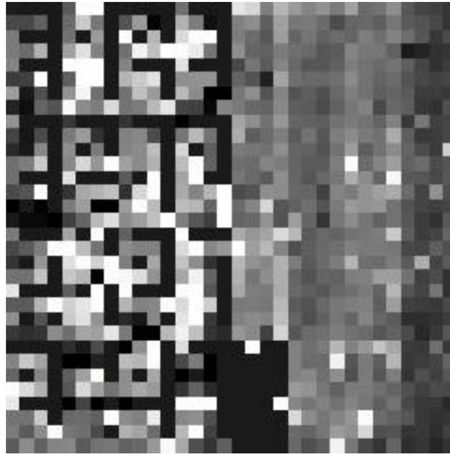
**Figure 5. Operation of the 70 Micron Array.** The scan mirror is in the "SED" position. Although this is the same measurement condition as the array images displayed in the reports for Campaigns D2 and E, that array now shows a fixed pattern of offsets on Side B. Many of the pixels on this side have been put below the negative rail of the ADC. Side A behaves as expected (except for the loss of readout 4,4).
